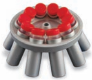
Ref. 1461-1744C 10x50 ml. Falcon Angular 30° Max. 4500 rpm. Max. 2830 xg.
