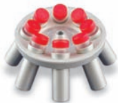
Ref. 1461-1213 8x50 ml. Falcon Angular 30° Max. 5000 rpm. Max. 4032 xg.
