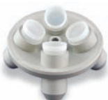
Ref. 1461-1718C 4x100 ml. Angular 30° Max. 5000 rpm. Max. 3158 xg.
